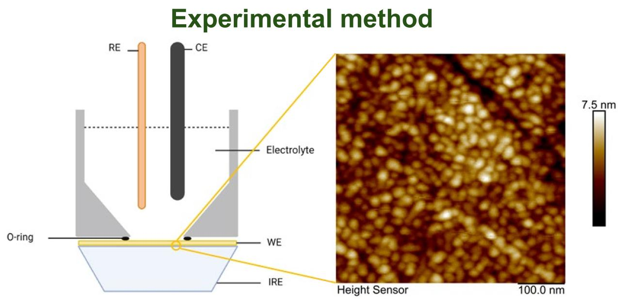
The experiments were conducted in three-electrode cell with a germanium crystal .Ag/AgCl was used as reference electrode I (RE) and graphite rod was used as the counter electrode (CE). 30 nm Cu was prepared by magnetron sputtering as working electrode (WE).
